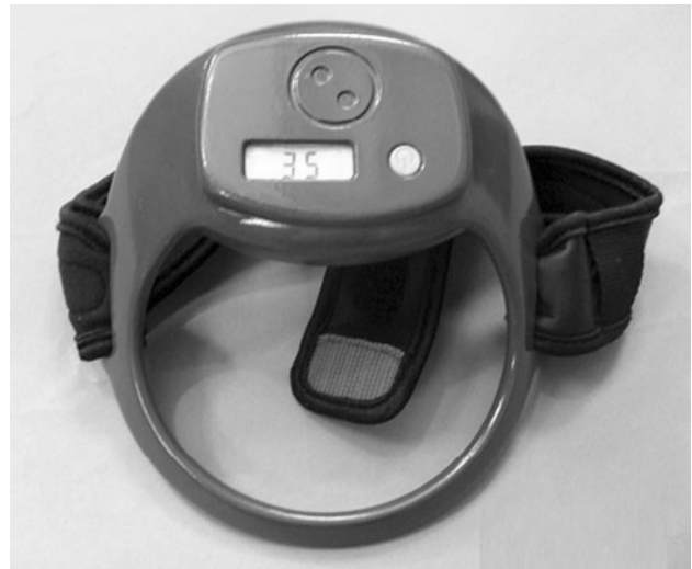
Fig. 1 The non-thermal pulsed radio frequency PEMF device used in this randomized, double-blind clinical study on knee OA pain. The device consists of a single loop wire coil with integrated amplifier (Palermo, Ivivi Health Sciences, San Francisco, CA) that delivers a PRF signal configured to modulate the CaM/NO/cGMP signaling pathway, which consisted of a 7-ms burst of a 6.8 MHz sinusoidal carrier repeating at 2 bursts/s, delivering a peak induced electric field amplitude of 34 \pm 8 V/m in the knee. The device is portable and easily positioned by the patient over the knee with the Velcro™ strap. The number displayed is the number of PEMF treatments
